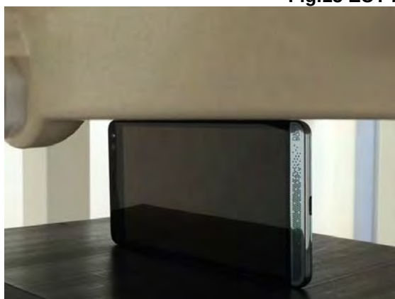
Fig.16 EUT right to flat phantom
