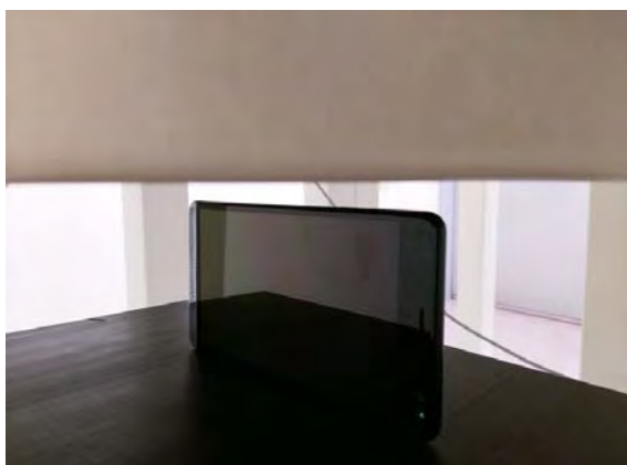
Fig.12 EUT Left side to flat phantom
