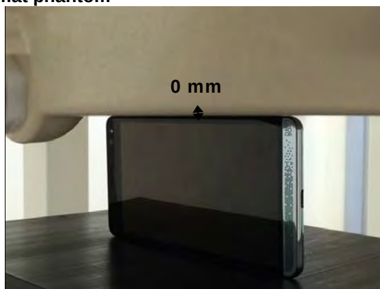
Fig.16 EUT right to flat phantom
