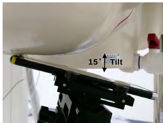
Fig.5 Right Head Section / Ear-Tilt Position(15°)
