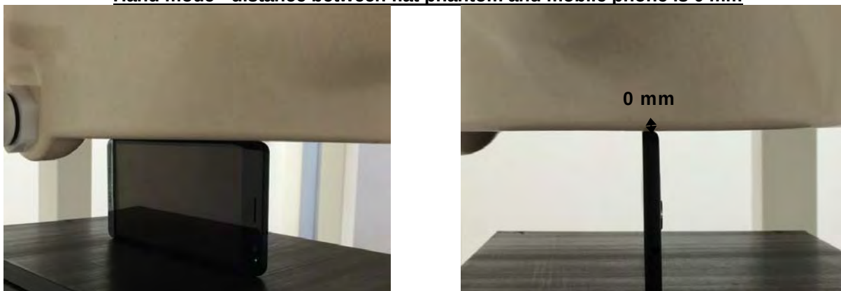
Fig.17 EUT left to flat phantom
