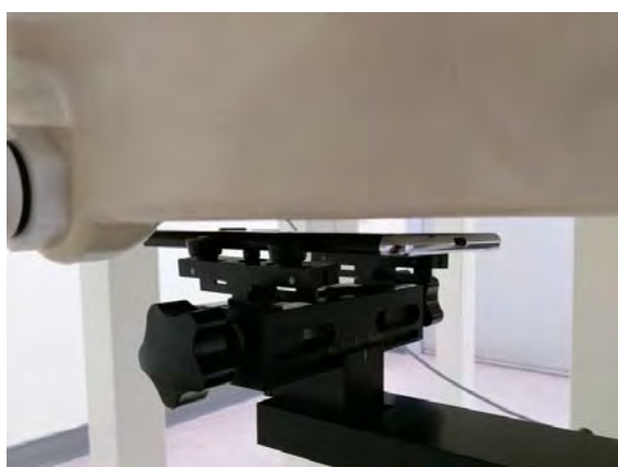
Fig.10 EUT Back side to flat phantom
