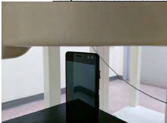
Fig.11 EUT Top side to flat phantom
