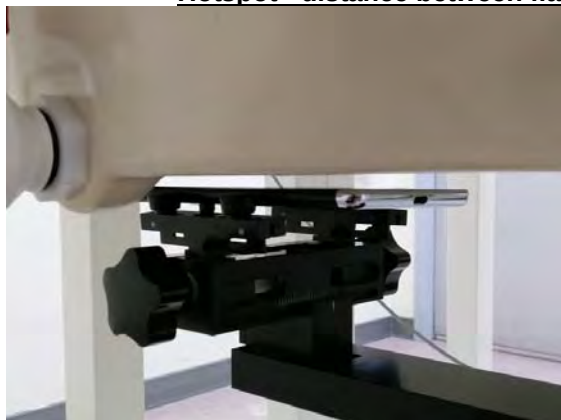
Fig.8 EUT Front side to flat phantom
