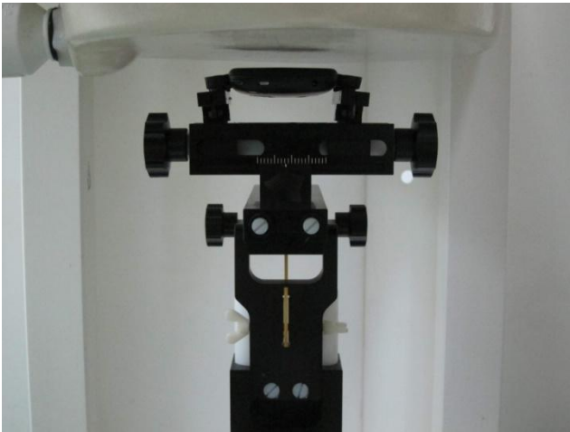
Front Face of the DUT with Phantom 1 cm Gap (DUT without Earphone)
