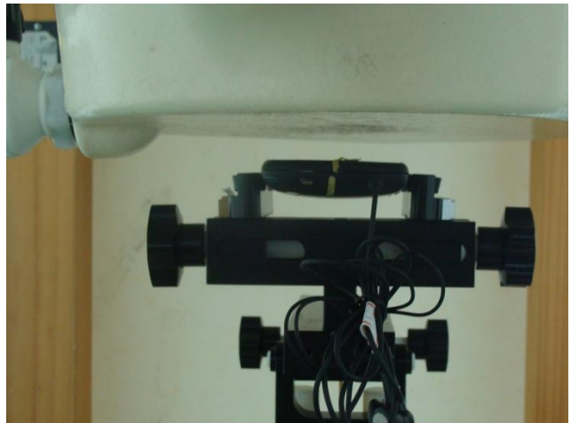
Front Face of the DUT with Phantom 1.5 cm Gap (DUT with Earphone)
