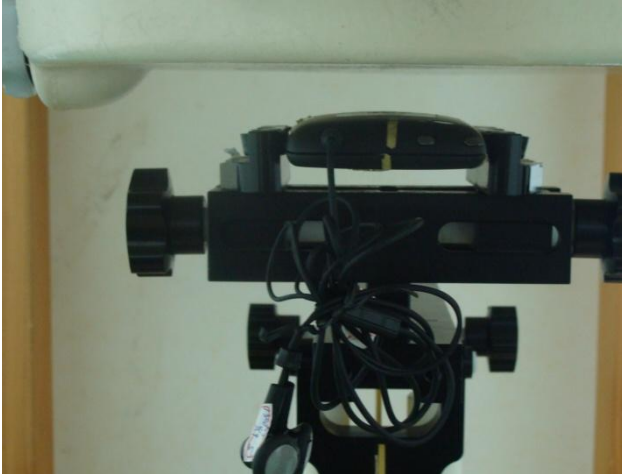
Rear Face of the DUT with Phantom 1.5 cm Gap (DUT with Earphone)
