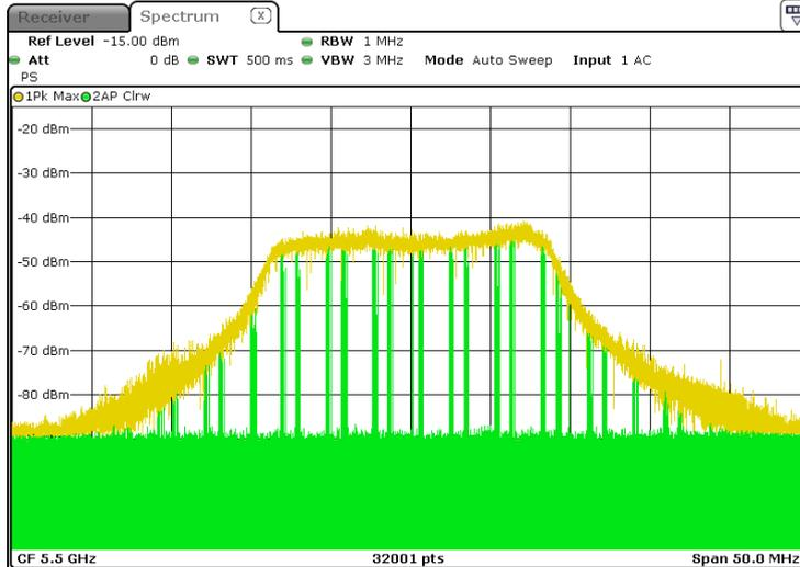
3) Radar signal 0 is applied to the Master device and WiFi traffic signal stop immediately.
