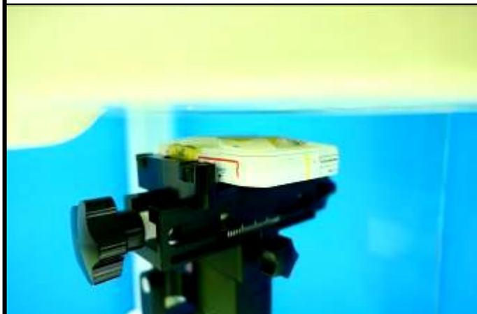
Rear Face of EUT at 13 mm
