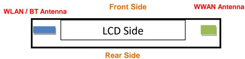
The separation distance for antenna to edge:
