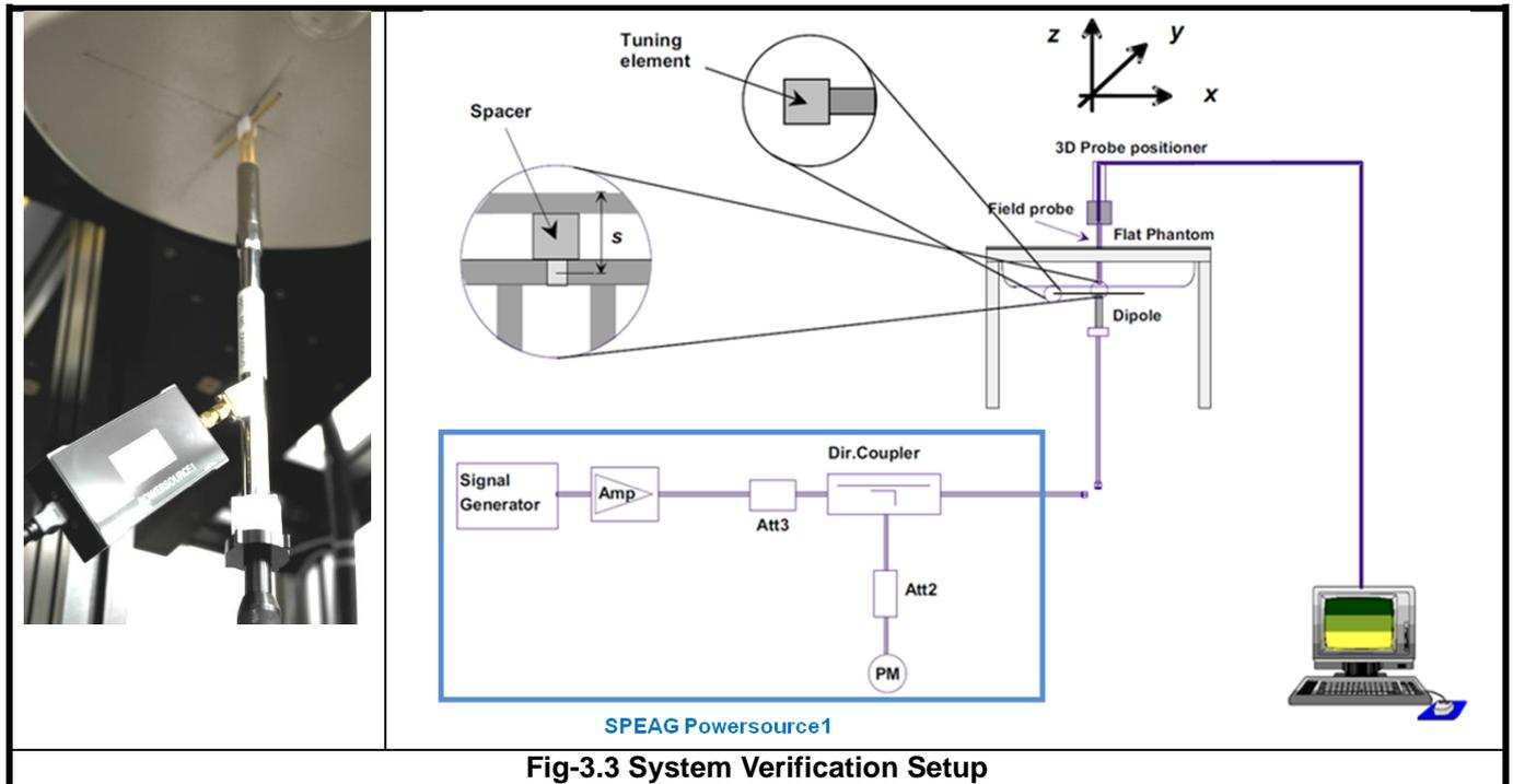
**Fig-3.3 System Verification Setup**
