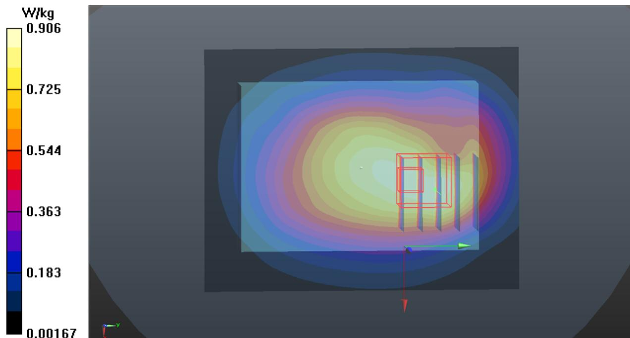
**P13 LTE 30\_QPSK10M\_Front Face\_5mm\_Ch27710\_1RB\_OS0\_P-sensor\_w**
