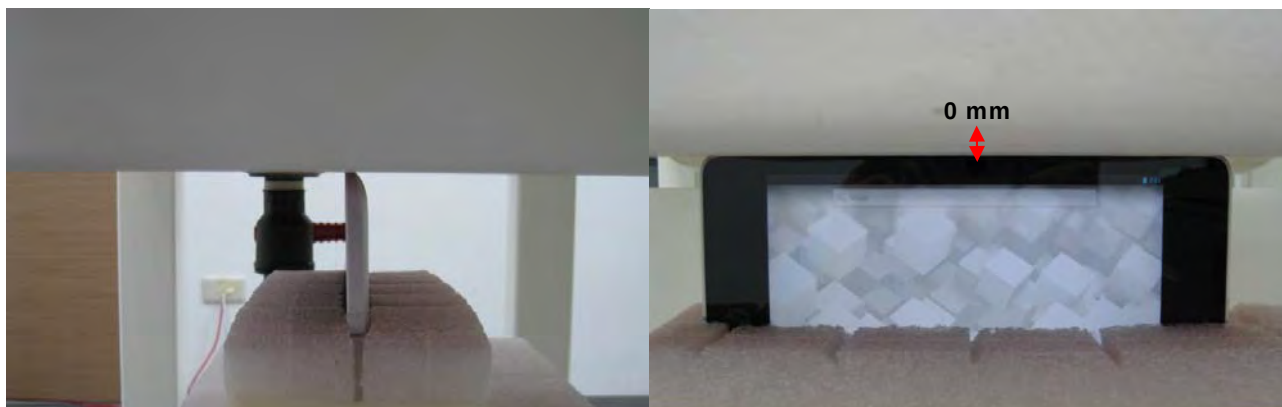
Fig.5 EUT Left side to flat phantom
