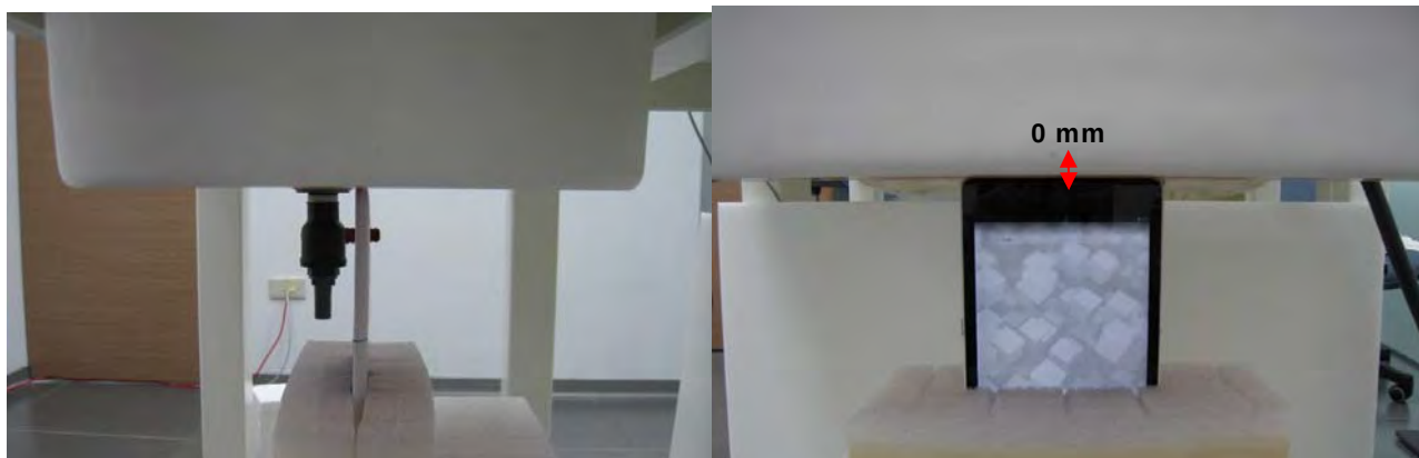
Fig.6 EUT Bottom side to flat phantom
