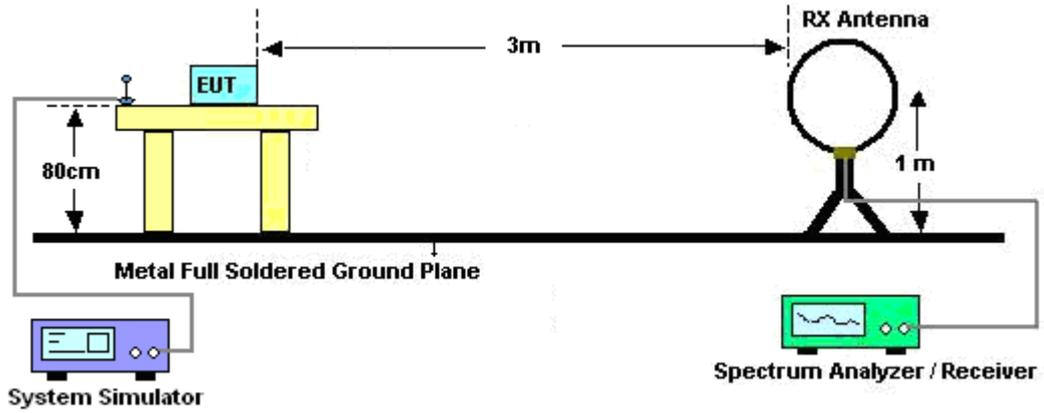
For radiated emissions from 30MHz to 1GHz
