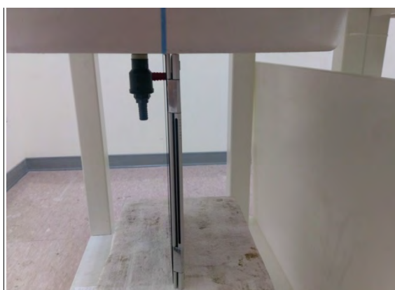
Fig.5 EUT Right side to flat phantom
