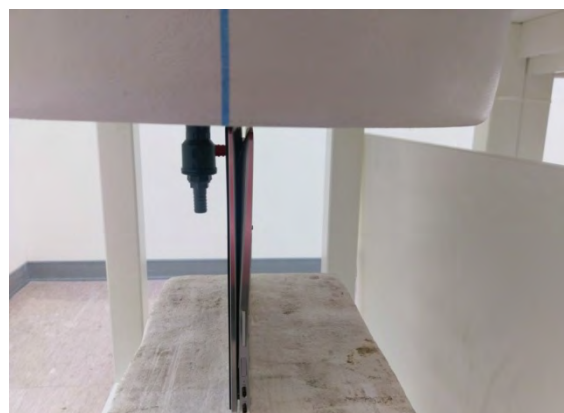
Fig.3 EUT Top side to flat phantom
