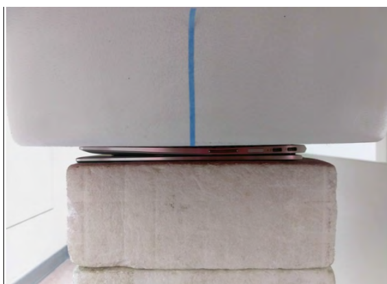
Fig.4 EUT Back side to flat phantom
