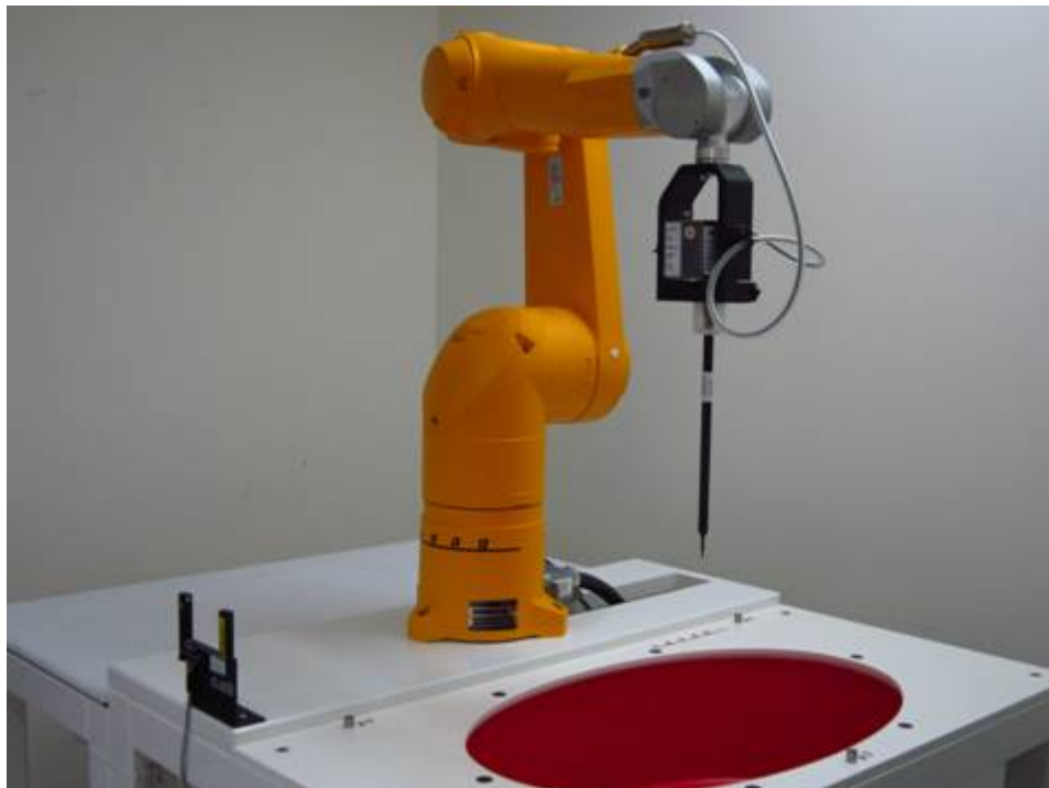
Fig.1 Photograph of the SAR measurement system
