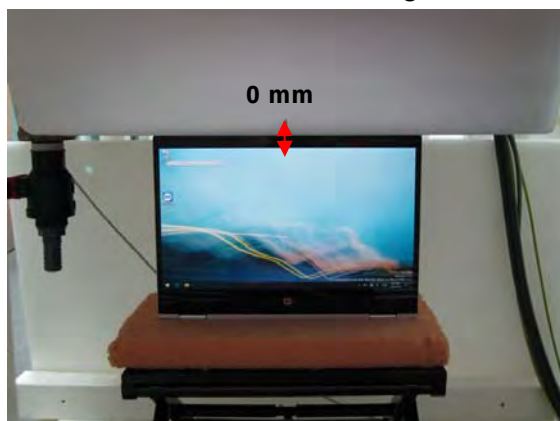
Fig.4 EUT Top side to flat phantom
