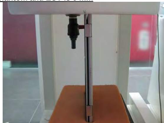
Fig.5 EUT Right side to flat phantom
