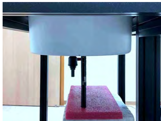
Fig.5 EUT Bottom side to flat phantom
