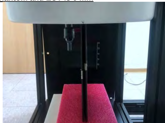
Fig.6 EUT Right side to flat phantom
