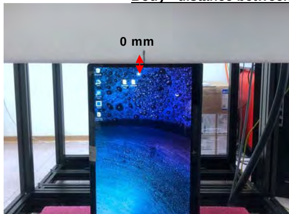
Fig.6 EUT Right side to flat phantom
