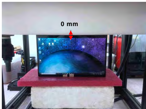
Fig.5 EUT Bottom side to flat phantom
