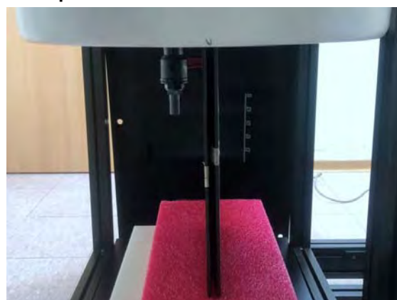
Fig.7 EUT Left side to flat phantom
