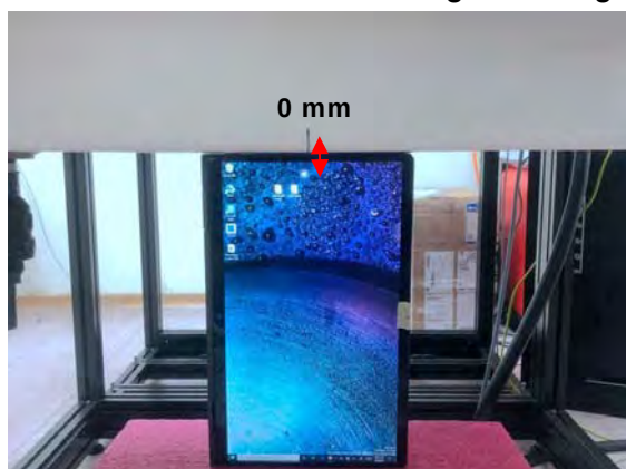
Fig.7 EUT Left side to flat phantom
