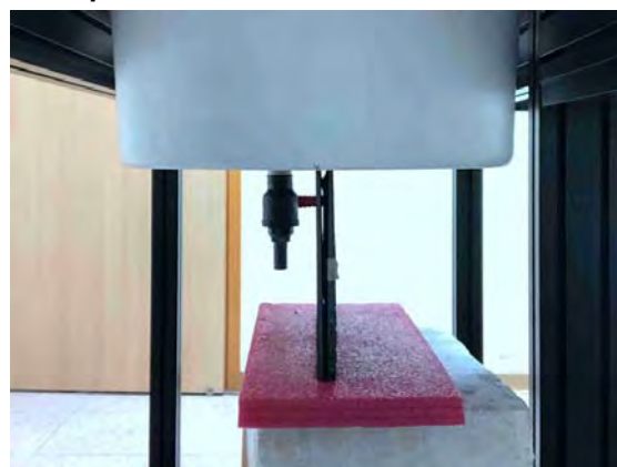
Fig.4 EUT Top side to flat phantom
