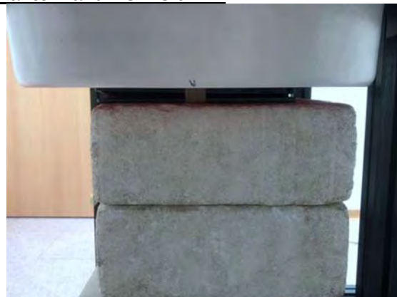
Fig.3 EUT Back side to flat phantom
