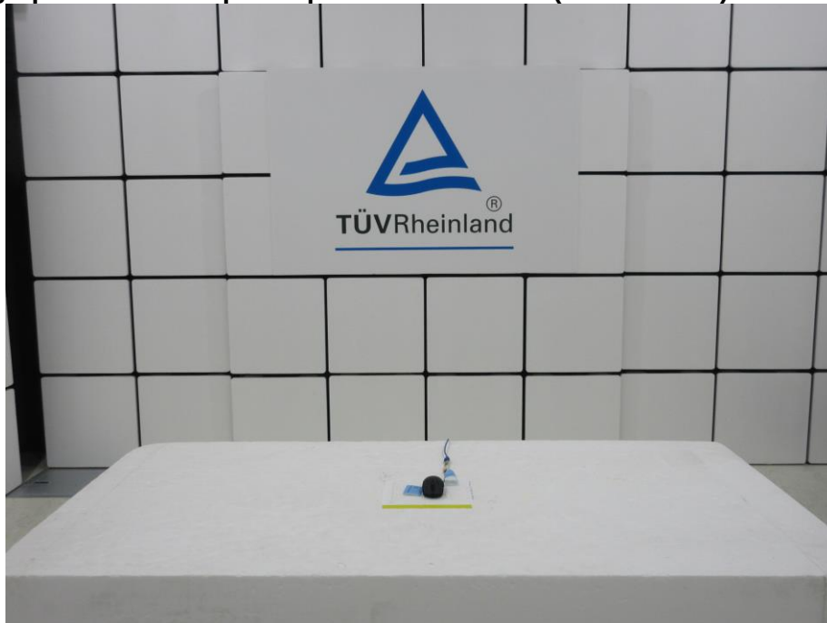
Photograph 2: Test Setup for Spurious Emissions (Front View 2)
