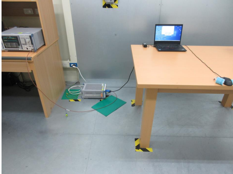
Photograph 15: Test Setup for Mains Conducted Emissions (Front View)
