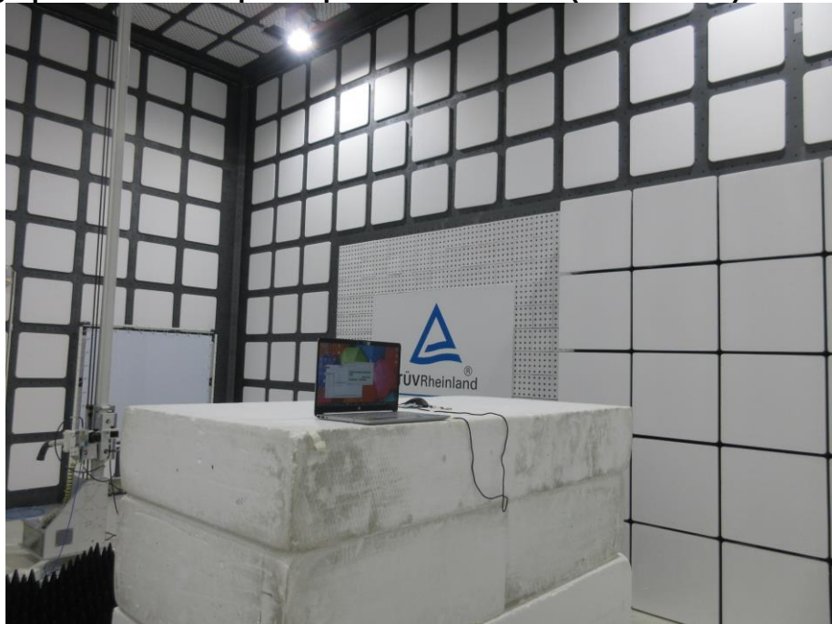
Photograph 14: Test Setup for Spurious Emissions (Back View 4)
