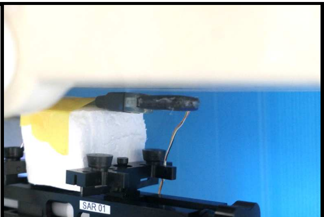
Horizontal Down of EUT Tested at 5 mm
