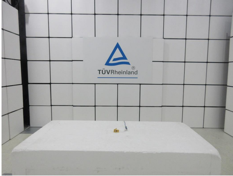
Photograph 2: Test Setup for Spurious Emissions (Front View 2)
