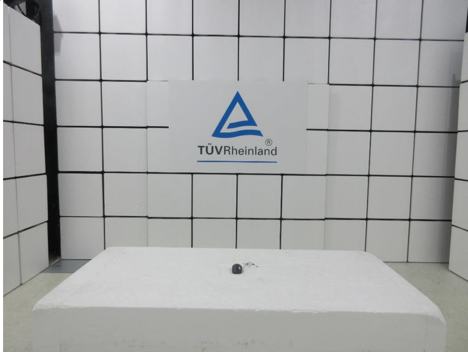
Photograph 1: Test Setup for Spurious Emissions (Front View 1)
