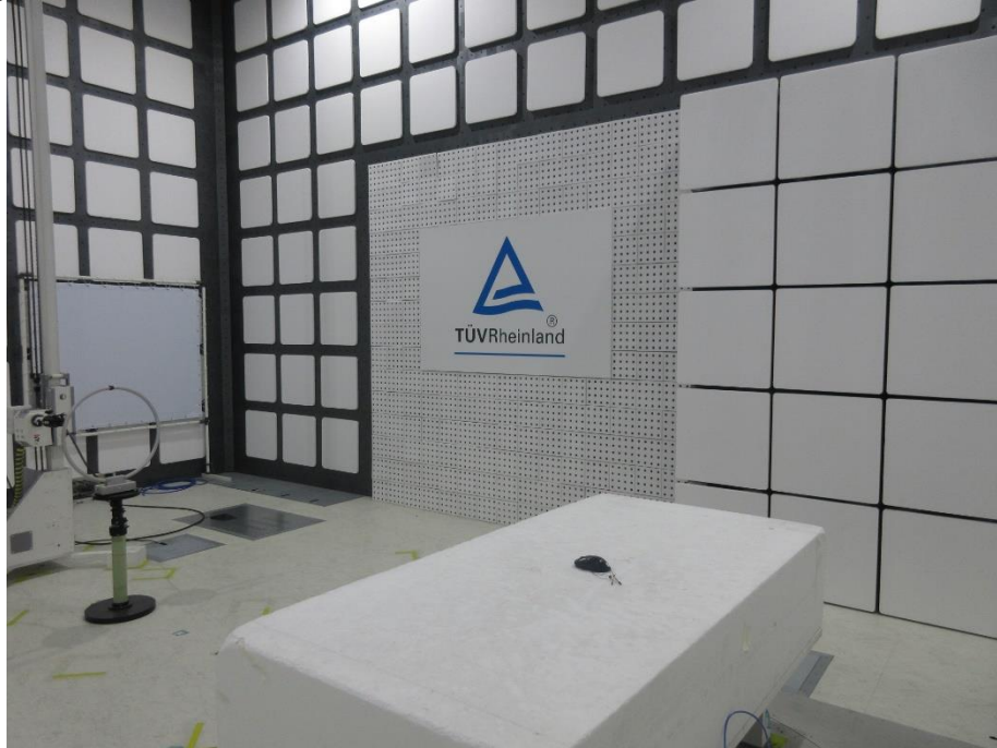
Photograph 3: Test Setup for Spurious Emissions (Back View 1)
