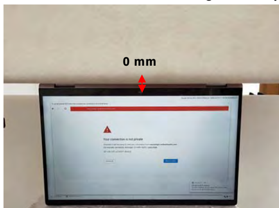
Fig.5 EUT Bottom side to flat phantom
