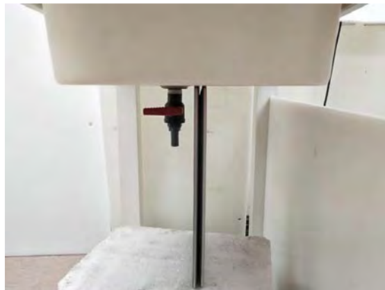
Fig.7 EUT Left side to flat phantom
