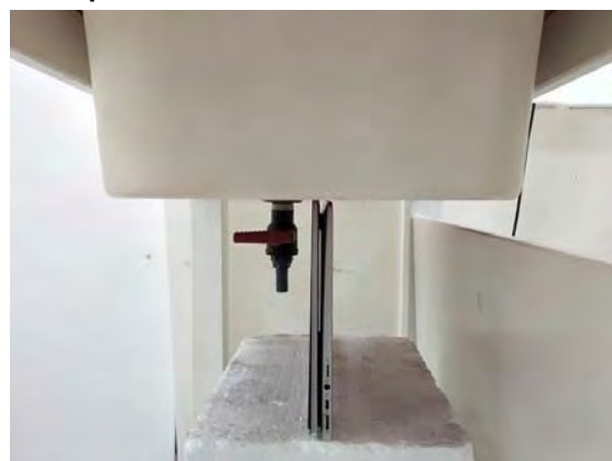
Fig.4 EUT Top side to flat phantom
