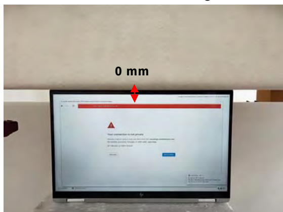
Fig.4 EUT Top side to flat phantom
