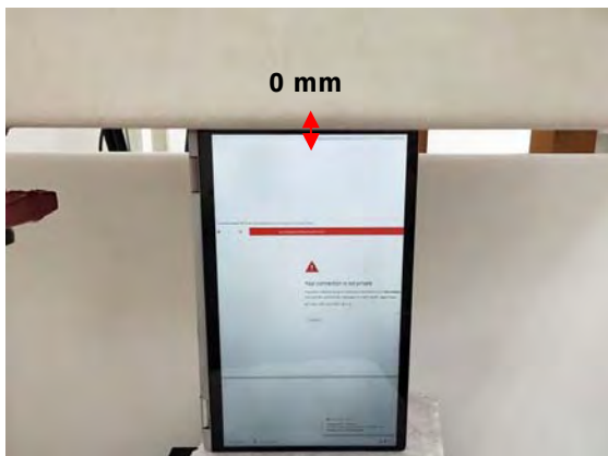
Fig.7 EUT Left side to flat phantom
