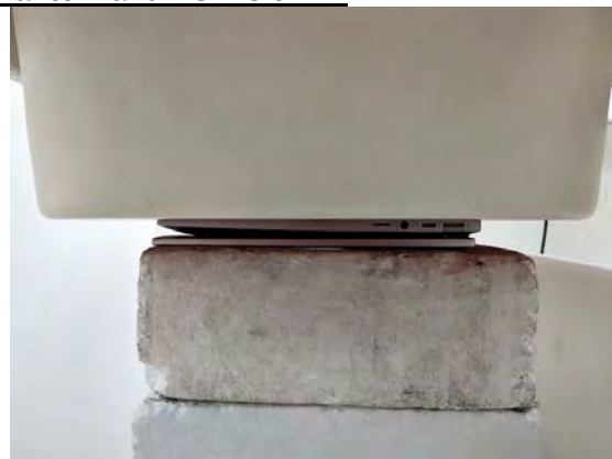
Fig.3 EUT Back side to flat phantom
