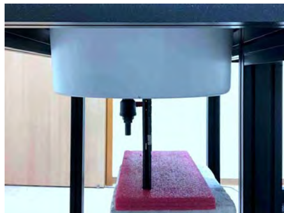
Fig.5 EUT Bottom side to flat phantom
