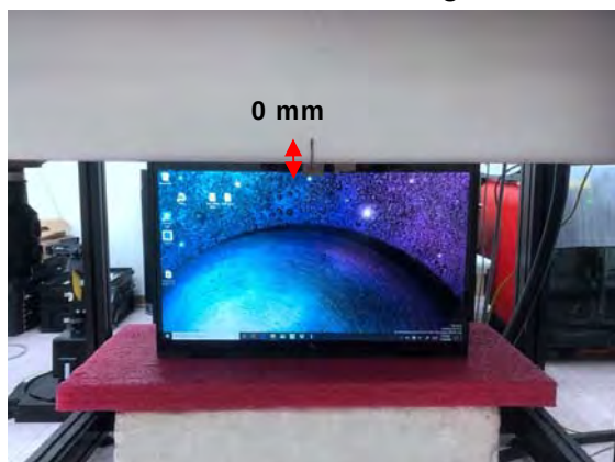
Fig.4 EUT Top side to flat phantom
