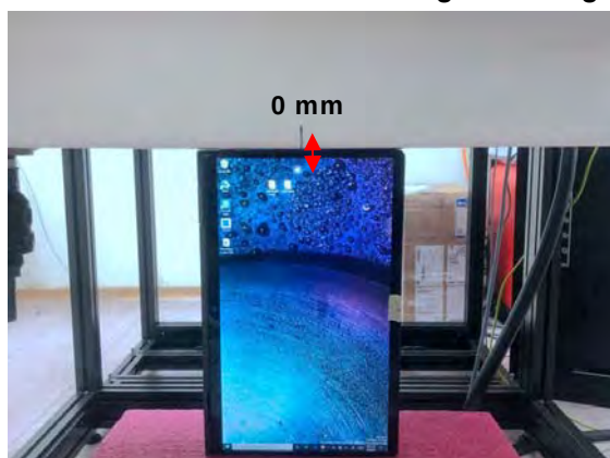
Fig.7 EUT Left side to flat phantom
