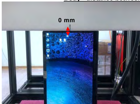
Fig.6 EUT Right side to flat phantom
