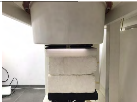
Fig.3 EUT Back side to flat phantom
