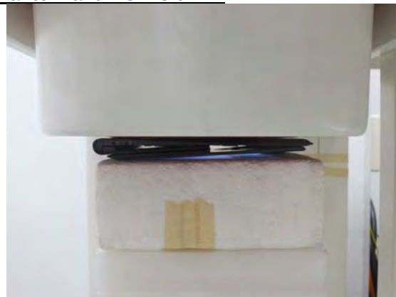
Fig.3 EUT Back side to flat phantom
