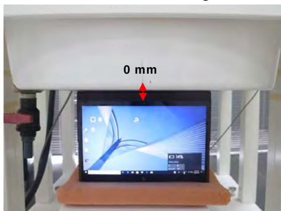
Fig.4 EUT Top side to flat phantom
