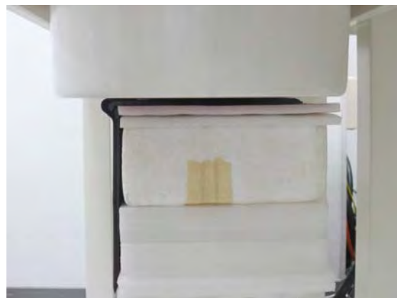
Fig.5 EUT Bottom side (Notebook mode) to flat phantom
