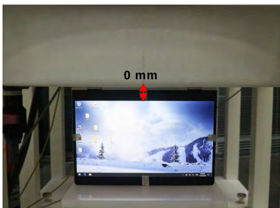
Fig.5 EUT Bottom side to flat phantom
