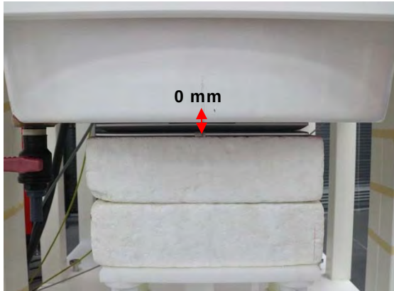
Fig.3 EUT Back side to flat phantom
