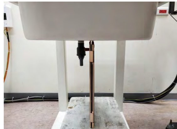
Fig.6 EUT Right side to flat phantom
