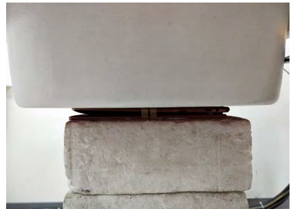
Fig.3 EUT Back side to flat phantom
