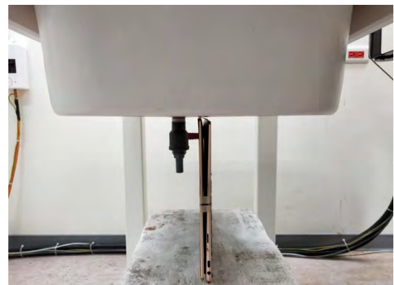
Fig.4 EUT Top side to flat phantom
