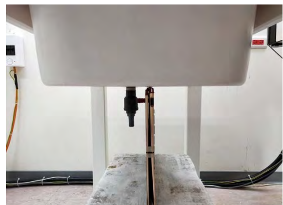
Fig.5 EUT Bottom side to flat phantom
