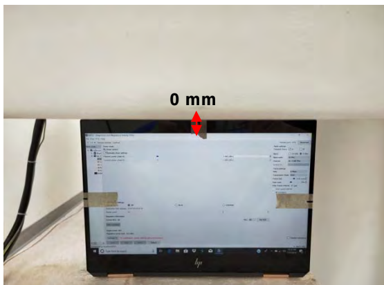
Fig.4 EUT Top side to flat phantom
