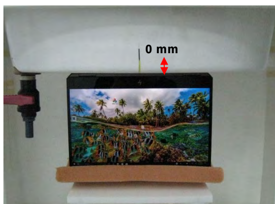
Fig.5 EUT Bottom side to flat phantom
