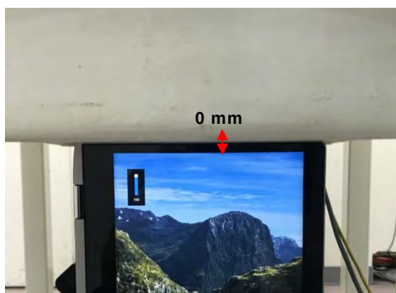
Fig.5 EUT Left side to flat phantom
