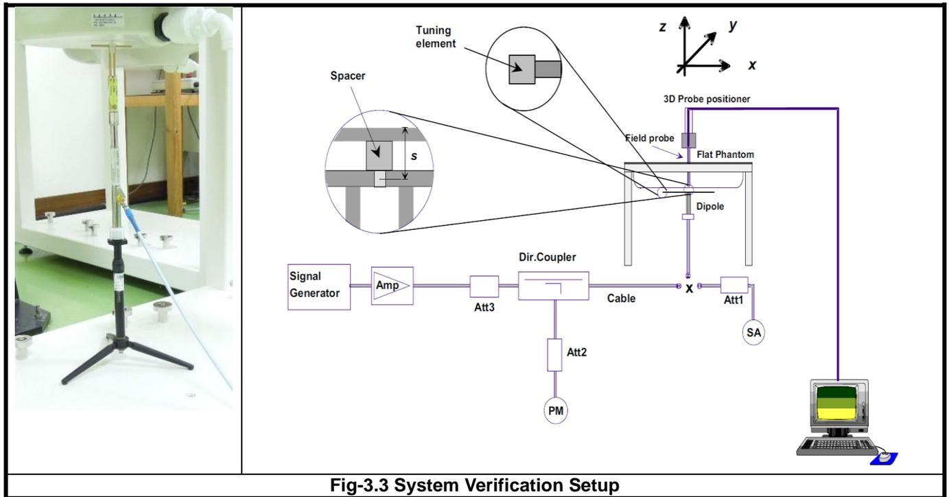
**Fig-3.3 System Verification Setup**
