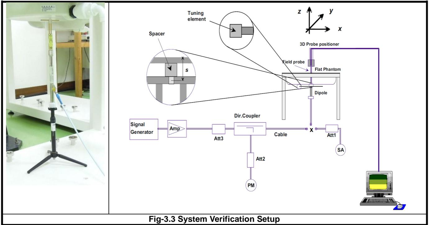
**Fig-3.3 System Verification Setup**
