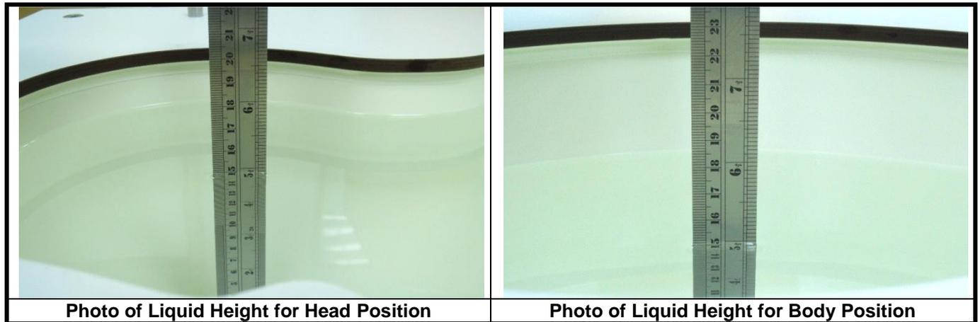
The dielectric properties of the head tissue simulating liquids are defined in IEEE 1528 and IEC 62209-1. For the body tissue simulating liquids, the dielectric properties are defined in RSS-102 Annex D and IEC 62209-2. The dielectric properties of the tissue simulating liquids were verified prior to the SAR evaluation using a dielectric assessment kit and a network analyzer.
