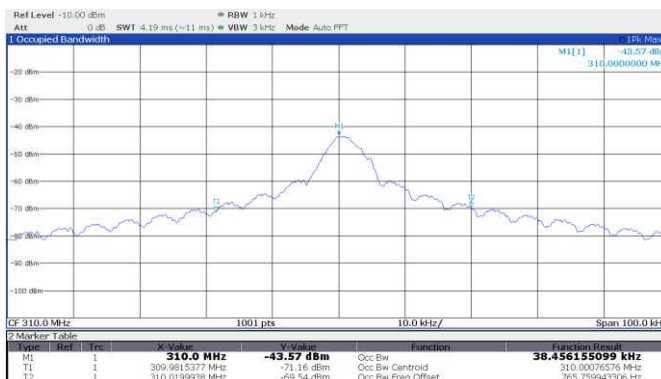
Figure 8.5-2: 99% occupied bandwidth, Sommer, rolling code, 310 MHz
