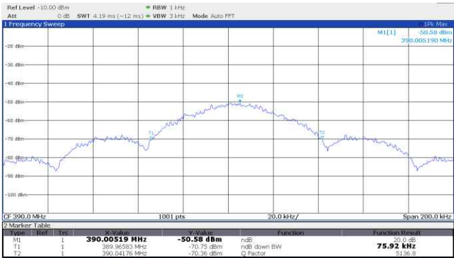
Figure 8.4-17: 20 dB bandwidth, Genie, 12 switch/2 position DIP switch, 1993-1995, 390 MHz
