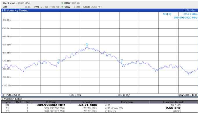
Figure 8.4-15: 20 dB bandwidth, Genie, Intellicode® II, 2010-2011, 390 MHz
