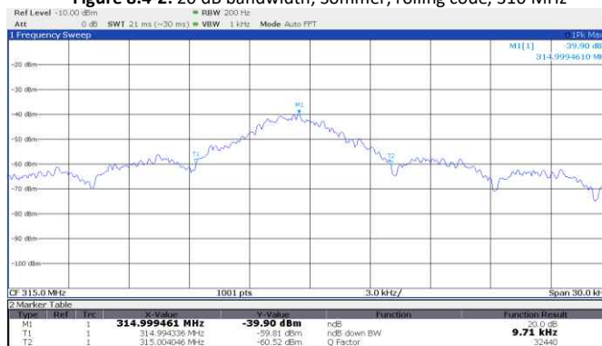
Figure 8.4-4: 20 dB bandwidth, Genie, Intellicode®, 1995-current, 315 MHz
