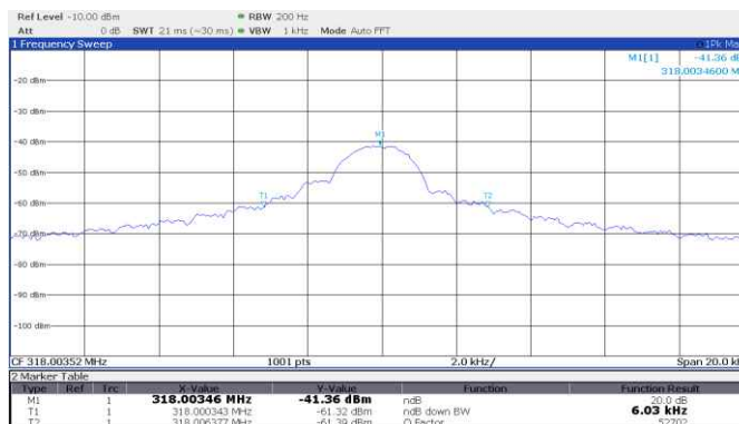
Figure 8.4-8: 20 dB bandwidth, Linear, Mega Code®, 318 MHz
