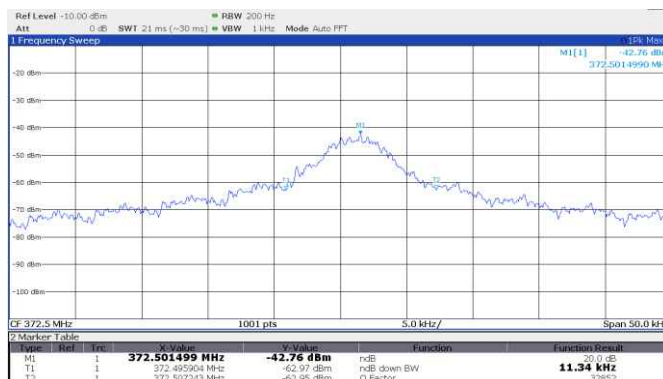
Figure 8.4-10: 20 dB bandwidth, Ryobi, rolling code, 372.5 MHz
