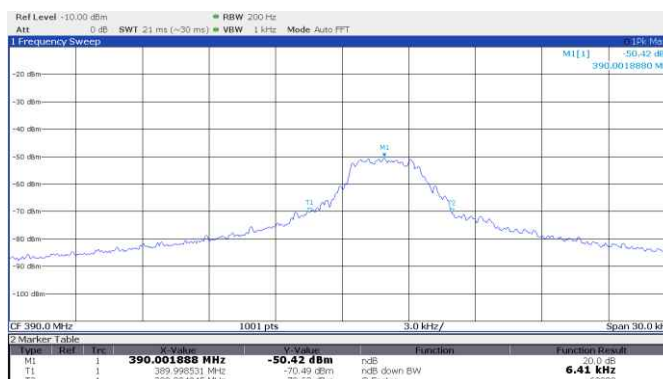
Figure 8.4-12: 20 dB bandwidth, Chamberlain, Orange/Red learn button, Security+®, 1996-2005, 390 MHz
