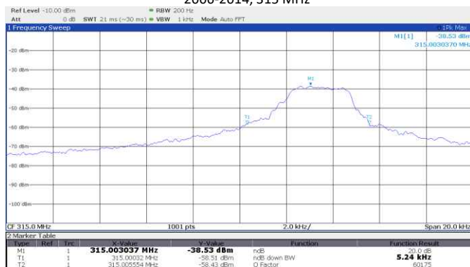
Figure 8.4-7: 20 dB bandwidth, Marantec, fixed learn code, 315 MHz
