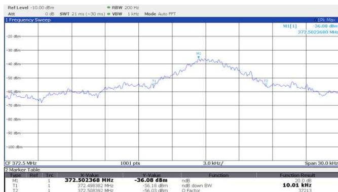
Figure 8.4-9: 20 dB bandwidth, Wayne Dalton, rolling code, 1999-current, 372.5 MHz
