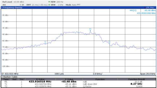
Figure 8.4-20: 20 dB bandwidth, FAAC, Rolling code, 433.92 MHz
