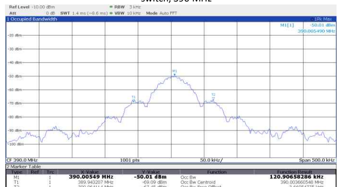
Figure 8.5-18: 99% occupied bandwidth, Genie, 9 switch/2 position DIP switch, 1993-1995, 390 MHz
