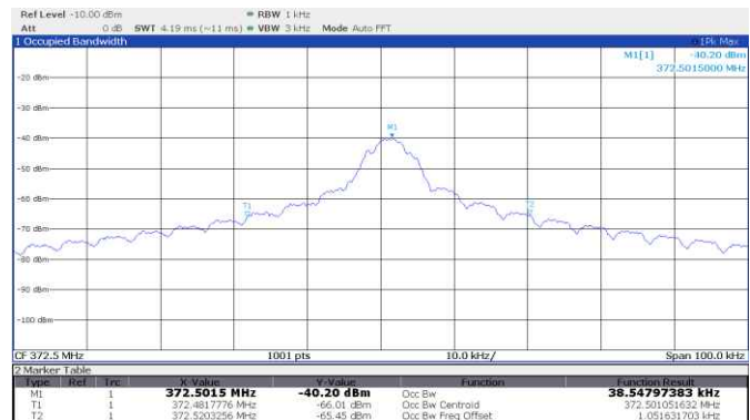
Figure 8.5-10: 99% occupied bandwidth, Ryobi, rolling code, 372.5 MHz
