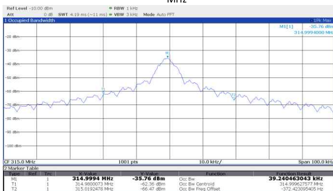
Figure 8.5-6: 99% occupied bandwidth, Genie, Intellicode® II, 2010-2010, 315 MHz
