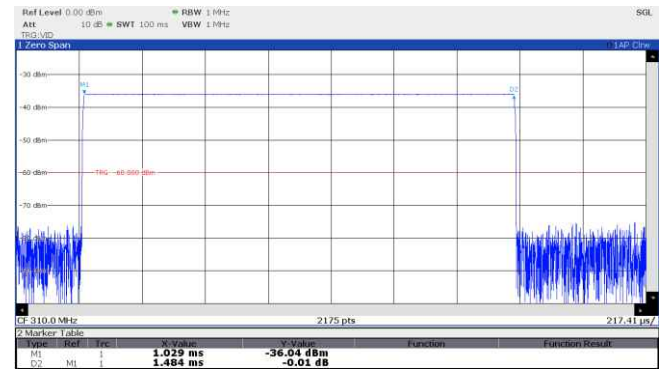
Figure 8.1-3: Duty cycle, Stanley, 10 switch / 2 position DIP switch, 310 MHz: 100 ms burst and pulse width measurements respectively
