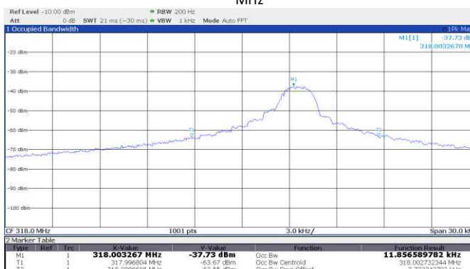
Figure 8.5-8: 99% occupied bandwidth, Linear, Mega Code®, 318 MHz
