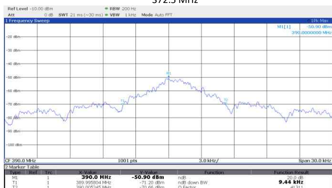
Figure 8.4-11: 20 dB bandwidth, Genie, Intellicode® I, 1995-current, 390 MHz
