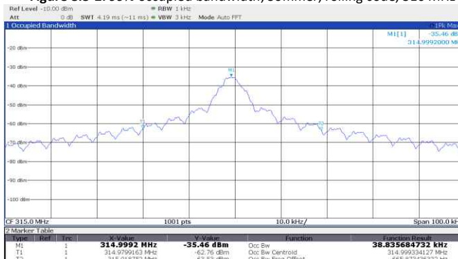
Figure 8.5-4: 99% occupied bandwidth, Genie, Intellicode®, 1995-current, 315 MHz
