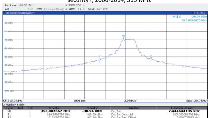
Figure 8.5-7: 99% occupied bandwidth, Marantec, fixed learn code, 315 MHz
