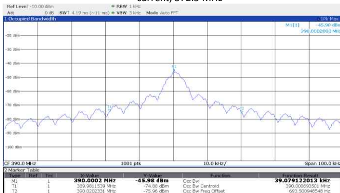
Figure 8.5-11: 99% occupied bandwidth, Genie, Intellicode® I, 1995-current, 390 MHz
