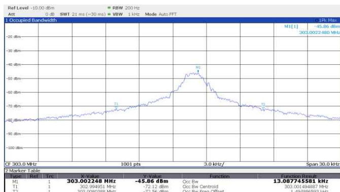
Figure 8.5-1: 99% occupied bandwidth, Guardian, fixed learn code, 303 MHz
