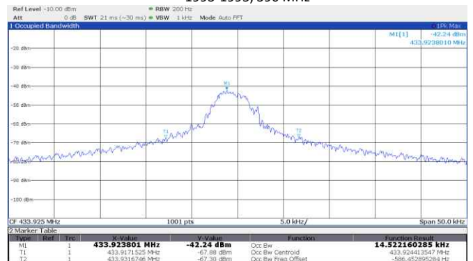
Figure 8.5-20: 99% occupied bandwidth, FAAC, Rolling code, 433.92 MHz
