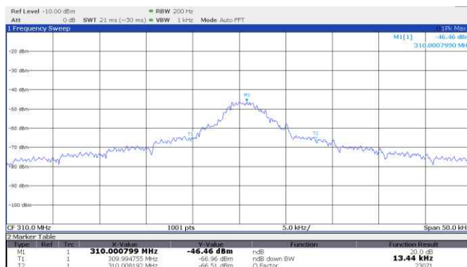
Figure 8.4-2: 20 dB bandwidth, Sommer, rolling code, 310 MHz
