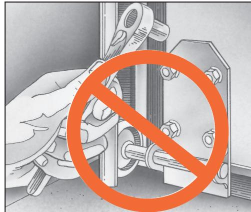
Never remove, adjust or loosen the screws on the bottom brackets of the door. These brackets are connected to the spring by the lift cable and are under extreme tension.
