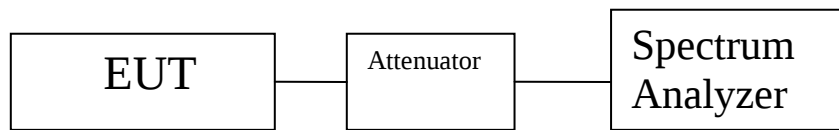
Figure 3. Block Diagram, Conducted Spurious Emissions Test Setup
