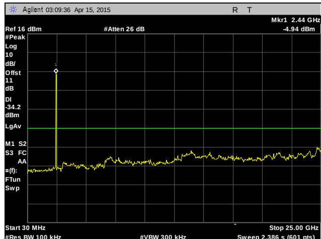
Plot 26. Conducted Spurious Emissions, High Channel, 30 MHz – 25 GHz
