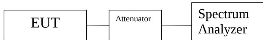
Figure 4. Block Diagram, Peak Power Spectral Density Test Setup
