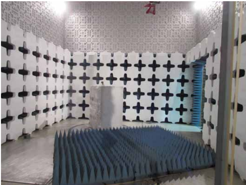
Test Setup for Radiated Emissions, 1 to 4.5GHz – Vertical Polarization
