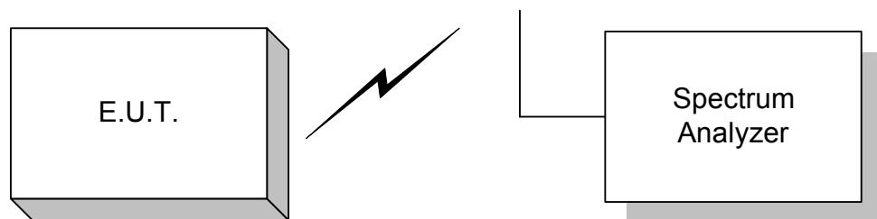
**Outdoor Test Site For Radiated Emissions**
