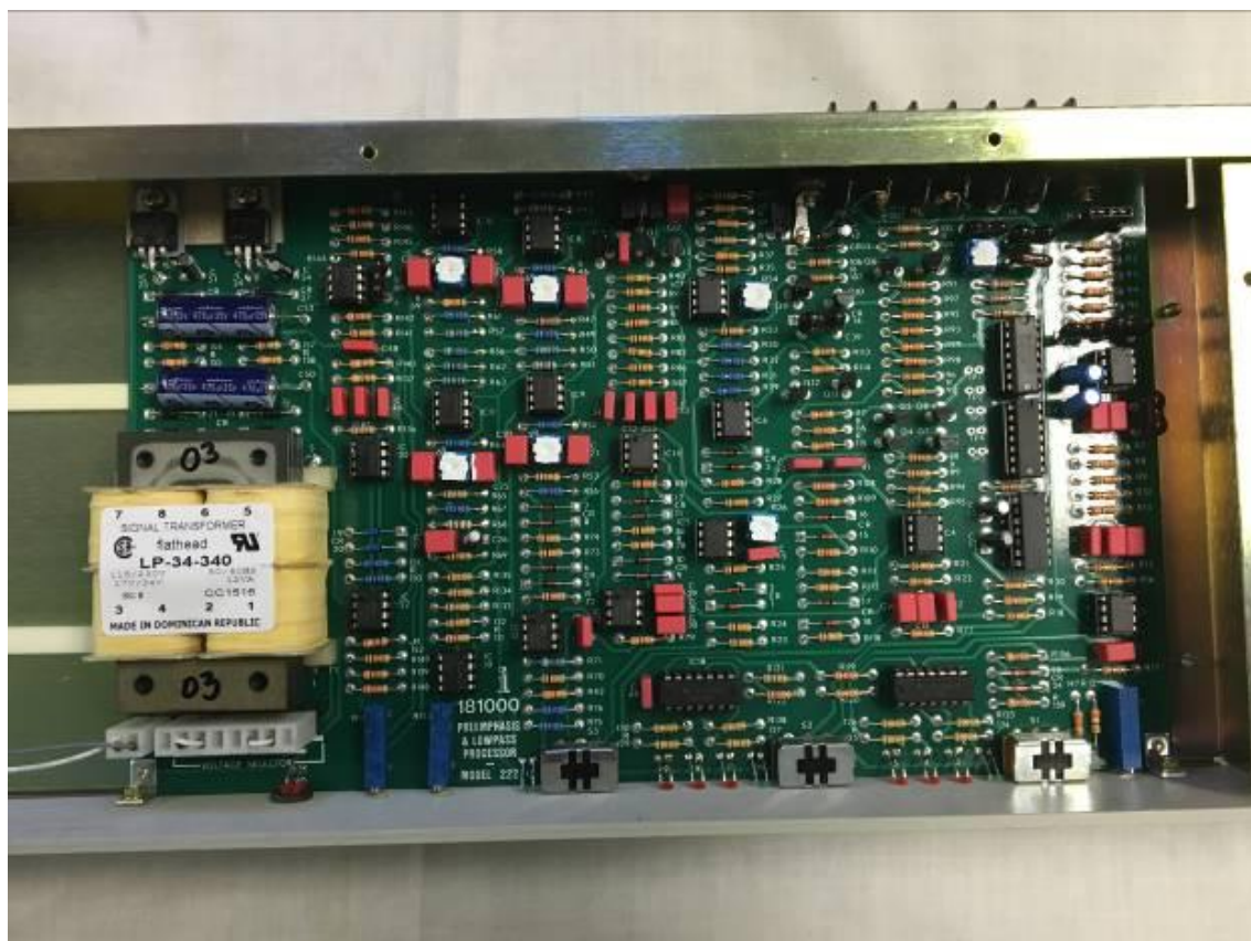
Figure 6. Filter #1 (Active) Main PCB
