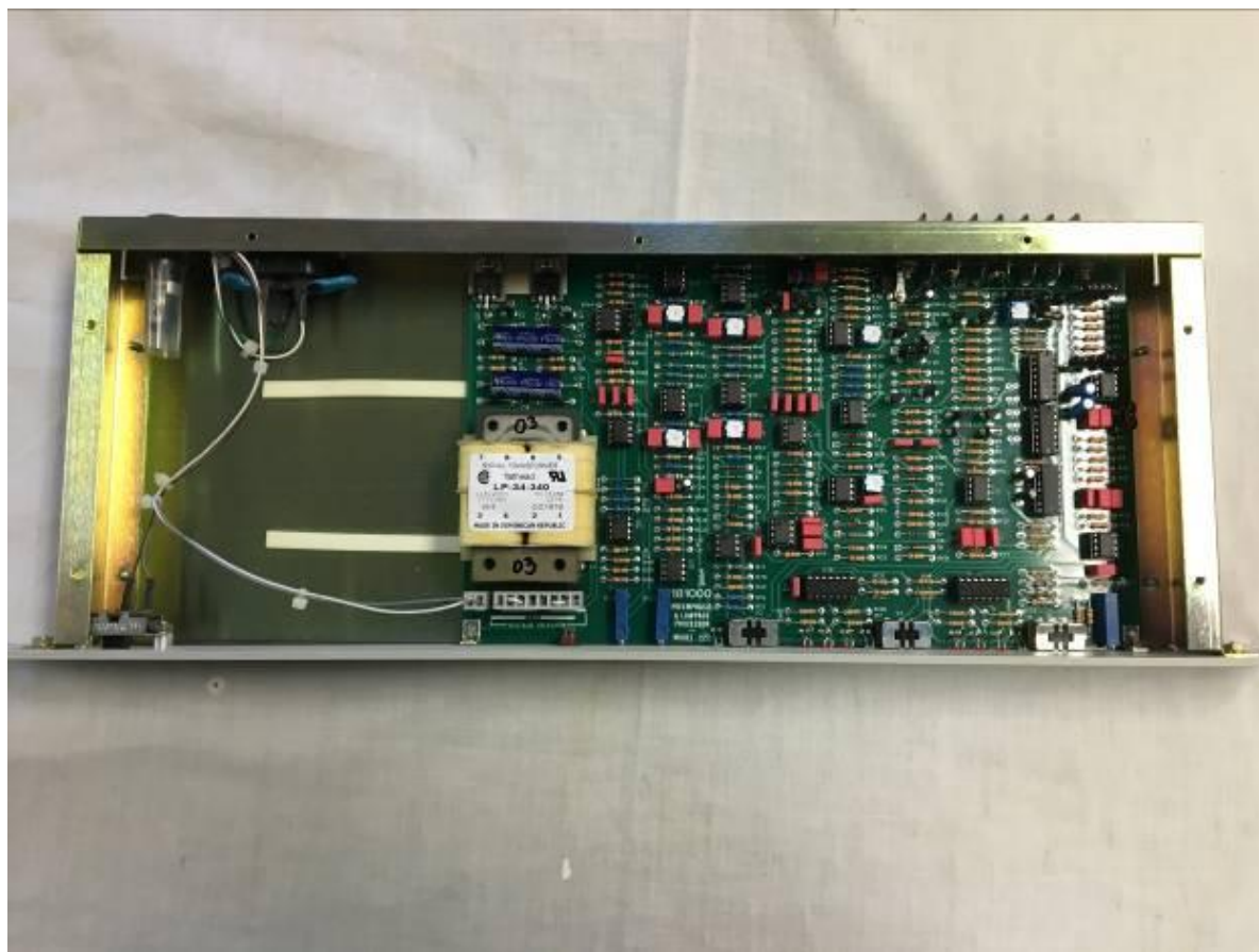
Figure 5. Filter #1 (Active) Top Cover Removed
