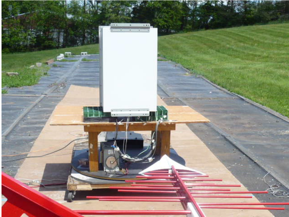
Horizontal Antenna Polarization, 30 MHz to 1 GHz
