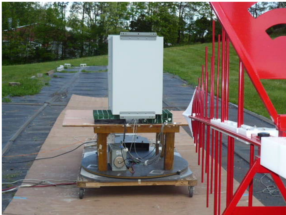
Vertical Antenna Polarization, 30 MHz to 1 GHz
