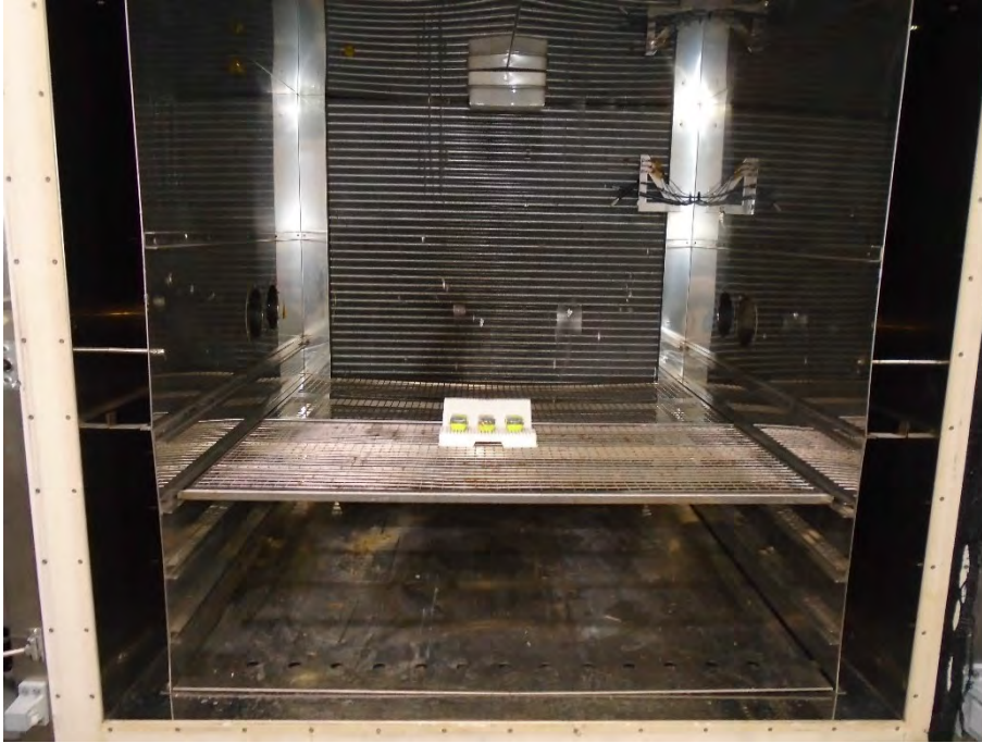
Test Setup – EUTs installed in climatic chamber
