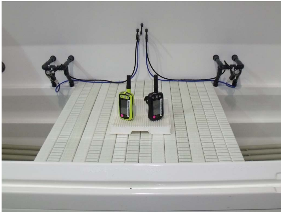
Spray Test Setup
