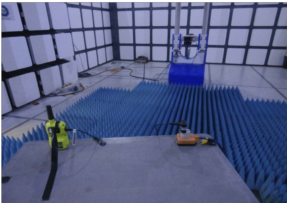
Figure 9 - Test Setup - > 1 GHz setup
