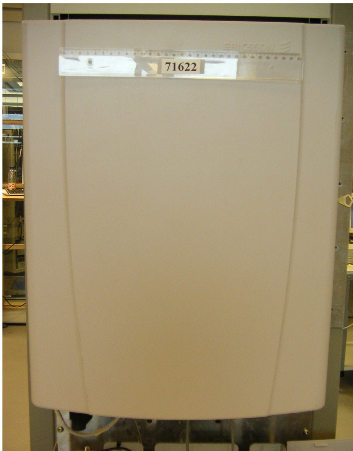
PHT/71622JD11/001 RBS2308 Cabinet with Shields and Mounting Base. Front View
