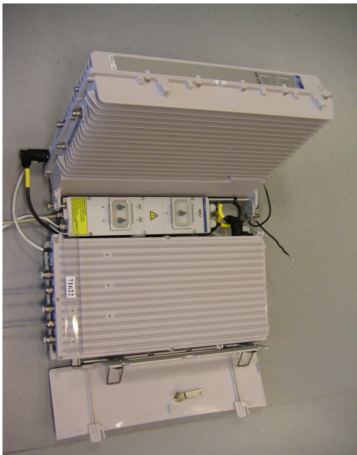
PHT/71622JD11/003 RBS2308 Cabinet with Mounting Base. Open View
