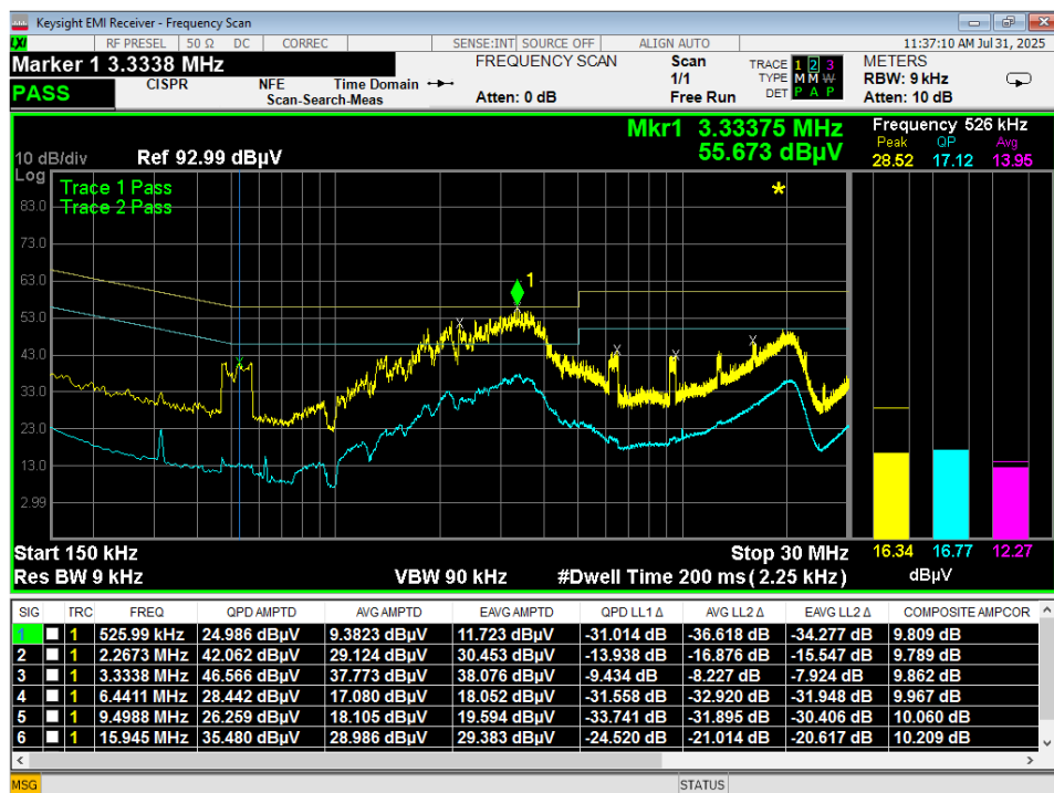
Figure 13 – Conducted Emissions Plot, AC Mains, IDLE, Line
