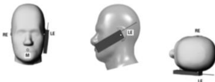
Front, Side and Top View of Cheek/Touch Position
