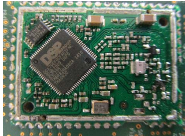
RF Module Cover Off View
