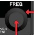
inner rotary Inner/Outer Rotary Encoder (right side)
