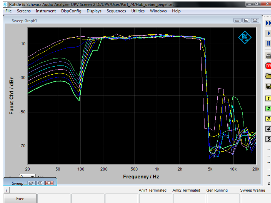
Plot 1: 10 curves with voltage and frequency variation 8.33 kHz
