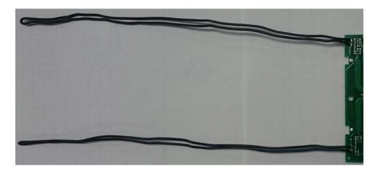
The antennas are made of stranded wire with black insulation with both ends soldered to PCB. The total length of each antenna is 22.4 cm. The design ensures that no antennas other than the one provided with the device shall be used with the intentional radiator.
