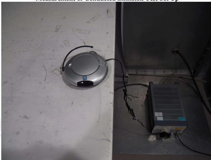
Measurement of Conducted Emission Test Set Up
