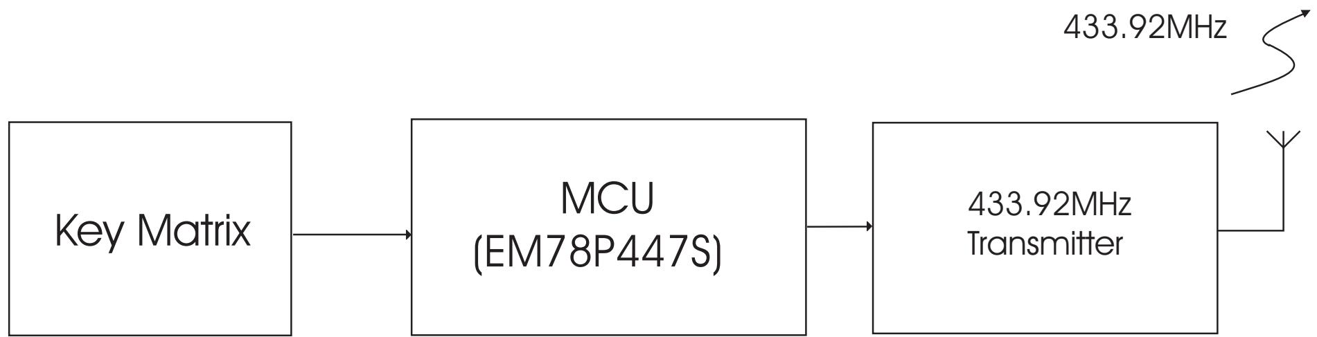
Block Diagram for SNAPSTREAM RF REMOTE (R1000)
