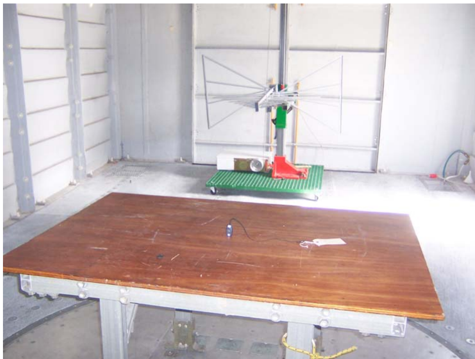
Radiated Emissions, Biconilog Horizontal Test Distance Setup
