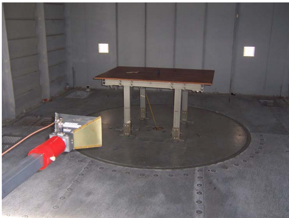
Radiated Emissions, Double Ridged Guide Vertical Test Distance Setup
