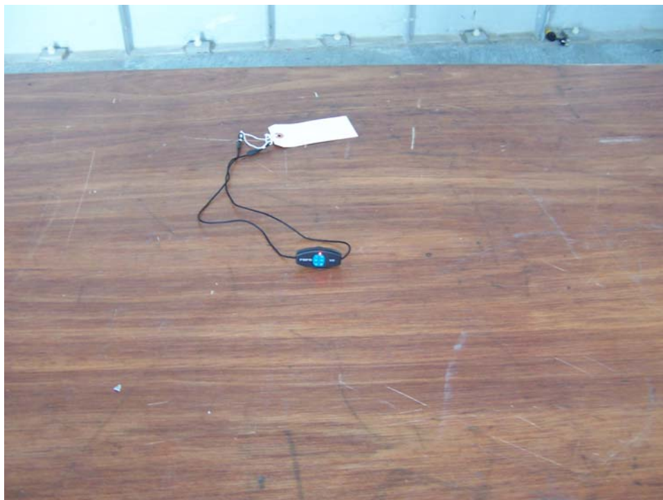
Radiated Emissions, Y-Axis Test Setup
