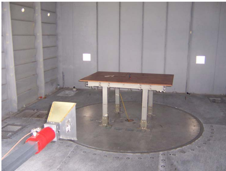
Radiated Emissions, Double Ridged Guide Horizontal Test Distance Setup
