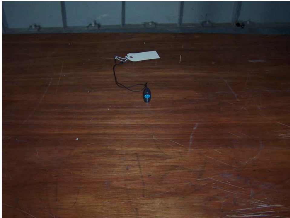
Radiated Emissions, Z-Axis Test Setup
